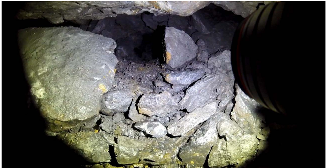
Photo 6. View of bottom of Borehole B-1 showing void area filled with collapsed material.
