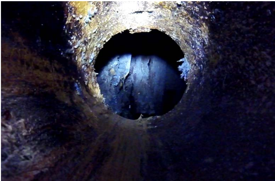
Photo 8. View through bottom of casing of Borehole B-3 showing fibrous wood debris.
