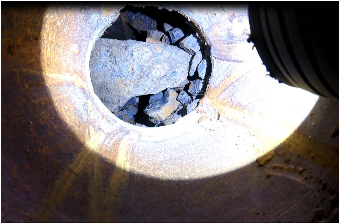
Photo 7. View through bottom of casing of Borehole B-2 showing void area filled with collapsed material.
